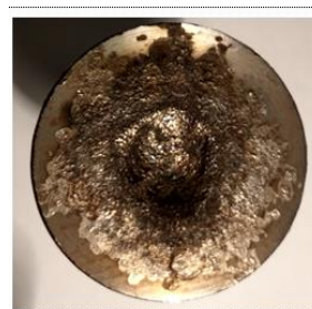
Figure 4 – Photograph of a sample with erosion according to these studies
