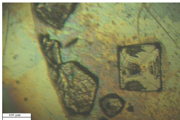
Figure 1 – Surface outgrowths after local treatment by solution
