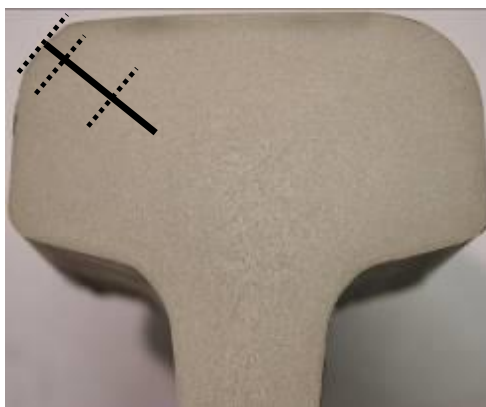
Figure 1 - Diagram of rail sample preparing on testing its structure by methods of electron diffraction microscopy. The direction along the fillet is designated with solid line; the regions of metal layers' location used for foil preparation are designated with dotted lines.
