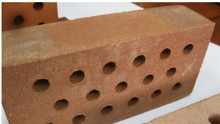
Figure 3. Ceramic brick on the basis of KCD class 40-80 mm enrichment waste of coaly argillites (sample of pilot lot produced at the Berdsky semi-dry pressing brick plant).
