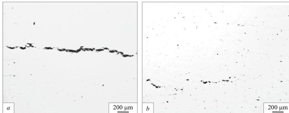
Fig. 3. The initial (a) and final (b) areas of an internal crack formed in the web of railroad rails.
