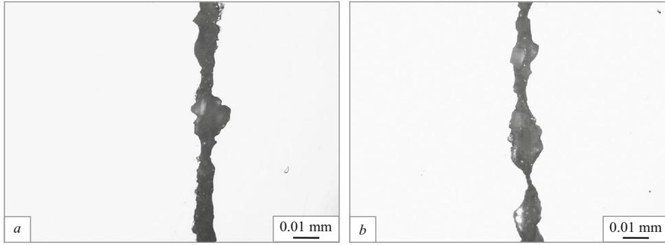
Fig. 1. The fragments of stratification in the web of railroad rails.
