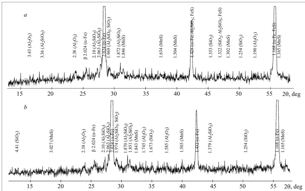
Fig. 2. Sections of diffraction patterns from the area of stratification localization in the rail web at the beginning (a) and end (b) of the defect.
