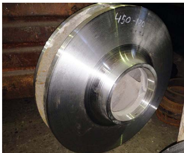
Figure 4. Responsible casting (rotor disk) without blown holes.
