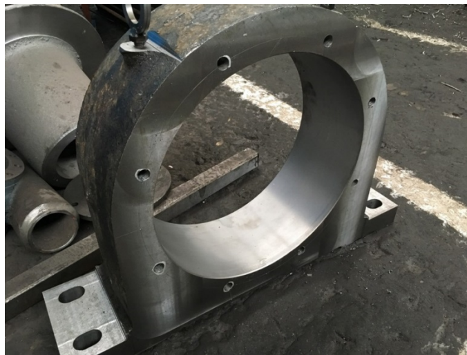
Figure 3. Casting (bearing housing) with effective metal deoxidation and heat-time treatment.
