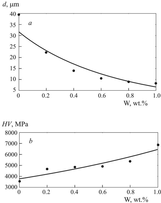
**Fig. 3.** Dependence of grain size (a) and cladding layer HV microhardness (b) on nanopowder tungsten concentration within cladding wire.
