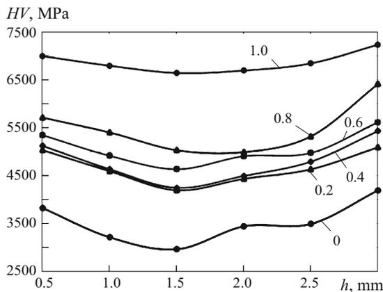
**Fig. 4.** Change in microhardness HV through cladding layer thickness within cross section ( $h$  is distance from surface). Figures on curves nanopowder tungsten content within cladding wire, wt.%.
