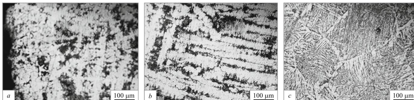
**Fig. 2.** Cladding and basic metal microstructure: a) region of “granular” dendrites; b) region of differently orientated dendrites; c) basic metal.
