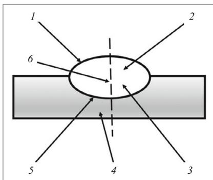
**Fig. 1.** Layout of test cladding layers areas: 1) cladding roller; 2) area of “granular” dendrites; 3) recrystallized dendrite region; 4) basic metal; 5) fusion zone of cladding roller and basic metal; 6) microhardness measurement line.
