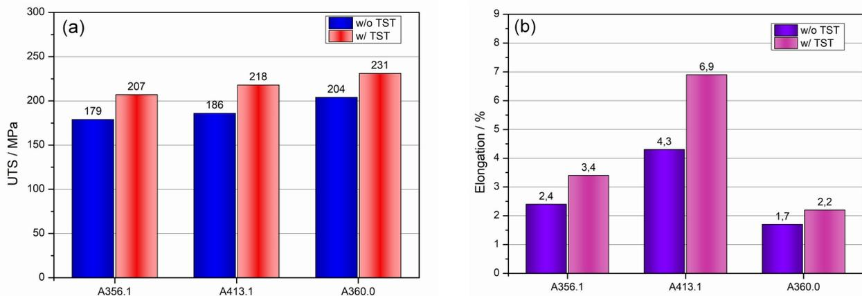
Fig. 2. Average values of ultimate tensile strength (*a*) and elongation (*b*) of aluminum alloys obtained by LFC-process with and without of TST
