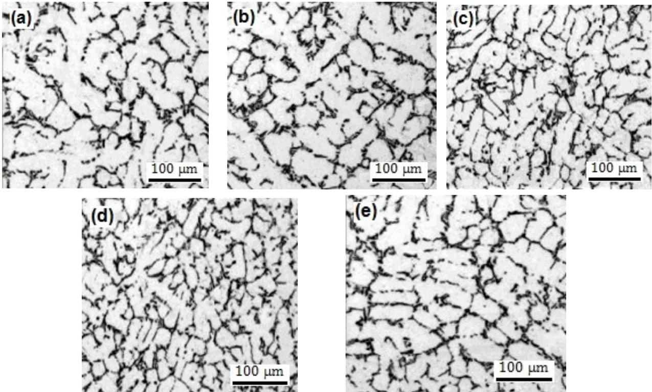
Fig. 1. Influence of the melt holding time during TST ( $\tau$ ) on the microstructure of castings from A356.1 alloy, obtained by LFC-process: *a*) initial alloy; *b*)  $\tau = 0...1$  min; *c*)  $\tau = 4...5$  min; *d*)  $\tau = 8...10$  min; *e*)  $\tau = 12...15$  min
