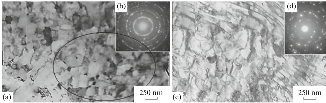
**Fig. 1.** Submicrocrystalline structure of (a, b) fillet and (c, d) tread surface of the rail head; ova in (a) indicates a region with a subgrain structure (ferrite grains are bright, cementite particles are dark).
