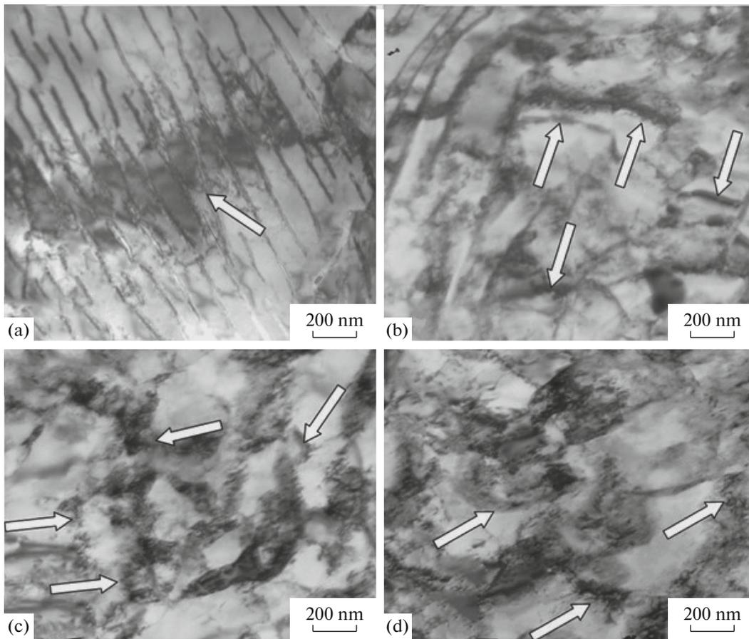
Fig. 2. Microstructure of the surface layer of the fillet (extinction bend contours are marked with arrows).
