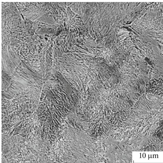
**Fig. 2.** Metal microstructure in the head of the investigated rail at a depth of 2 mm. Scanning electron microscopy of an etched section.
