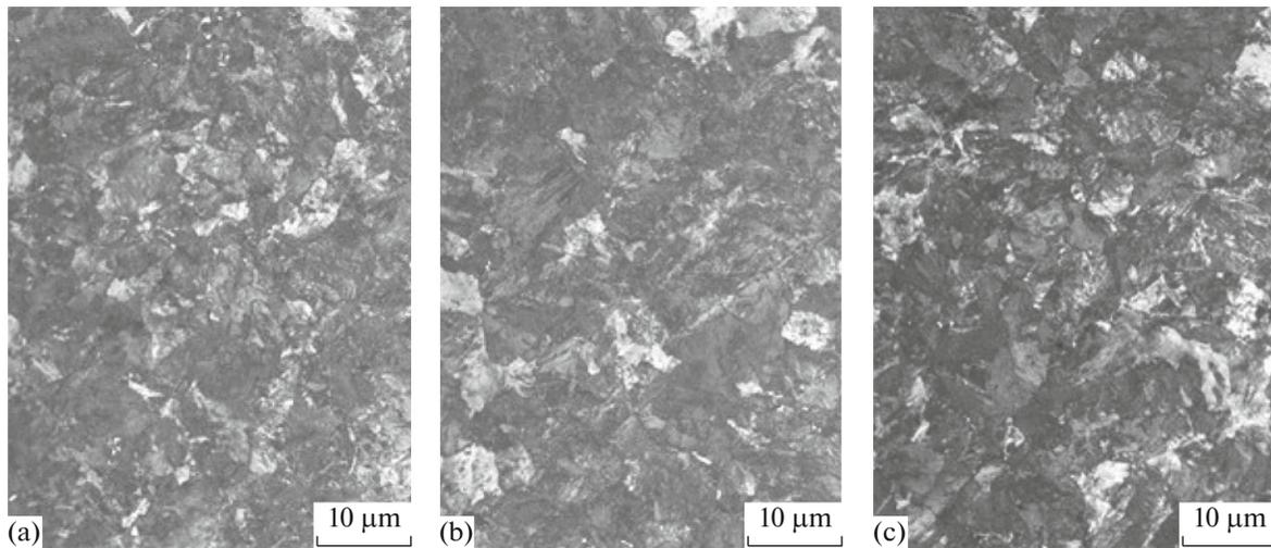
**Fig. 1.** Microstructure of the metal in the head of the investigated rail at a depth of 2 (a), 5 (b) and 10 mm (c) from the tread surface along the vertical axis.
