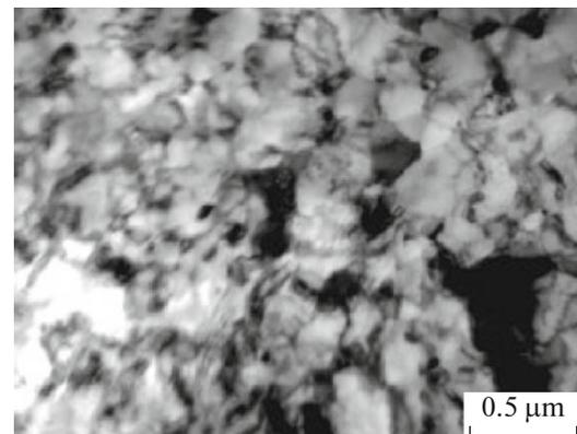
Fig. 4. Fragmented (subgrain) structure formed in the surface layer of the rail head metal.
