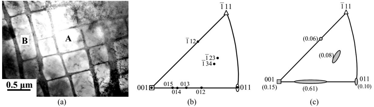
**FIGURE 1.** Original state of the Ni-Al-Co superalloy: (a) TEM image of the quasi-cuboidal structure (*A*—isotropic quasi-cuboids; *B*—anisotropic quasi-cuboids); (b) standard stereographic triangle with the indication of orientations; (c) orientations in the superalloy (dark regions) and their specific weight
