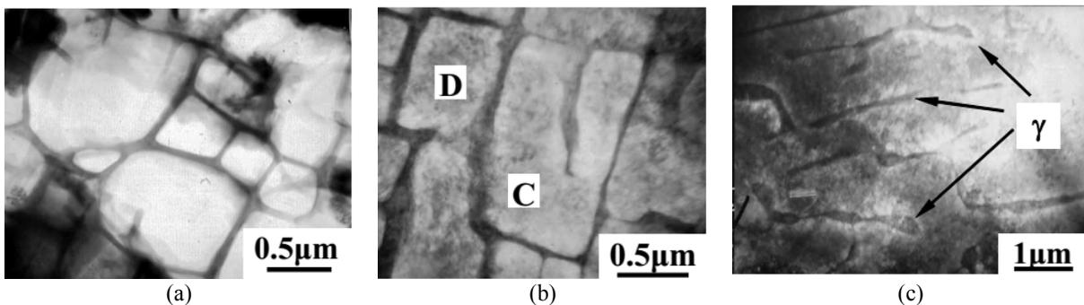
**FIGURE 4.** Quasi-cuboid morphology of the  $\gamma'$ -phase: (a) heterogeneous structure; (b) distorted structure (C—torn boundary, D—without a wall); (c) destructed (black arrows indicate individual walls)
