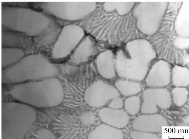
**Fig. 2.** Structure of silumin layer located at the depth of about 30  $\mu\text{m}$  after irradiation by electron beam ( $25 \text{ J/cm}^2$ ,  $150 \mu\text{s}$ , 3 pulses) [35].
