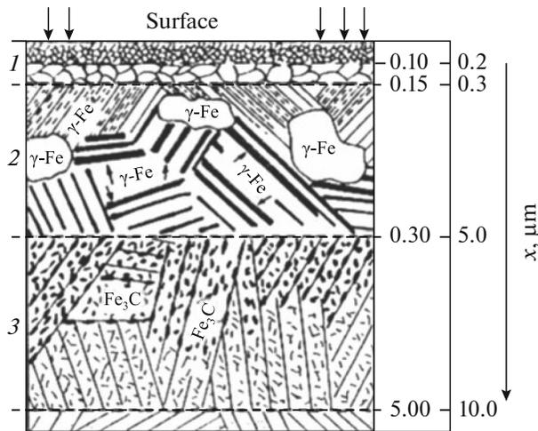
**Fig. 1.** Schematic view of pre-quenched steel 45 modified by electron beam (duration of electron beam pulse: 0.8  $\mu$ s, energy density: 2.2 J/cm<sup>2</sup>) [32].
