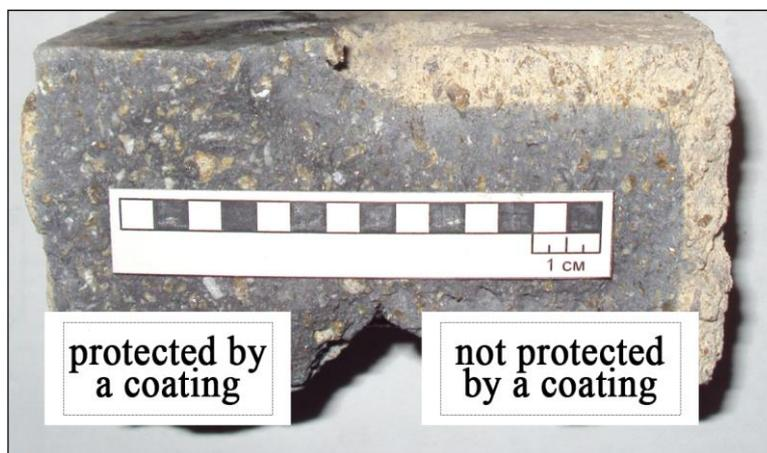
Fig. 2. Cross section of brick, the left half of which was protected by the coating, but the right half was in direct contact with oxidizing atmosphere.
