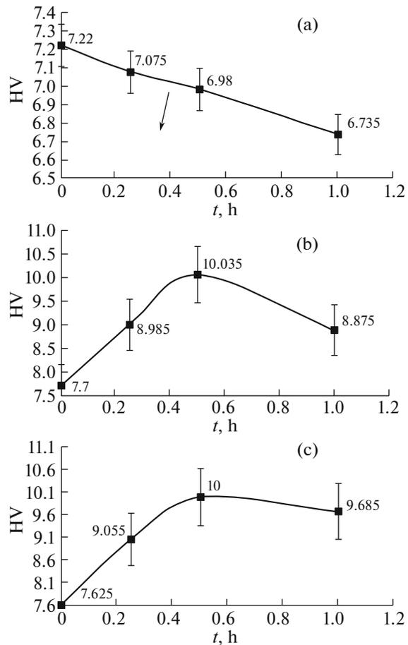
Fig. 3. Microhardness HV vs. The exposure time in the range from 0 to 1 h.  $B =$  (a) 0.3, (b) 0.4, and (c) 0.5 T.
