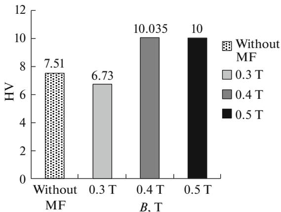
**Fig. 4.** Dependences of microhardness HV on the use of magnetic field and the values of induction  $B$ .
