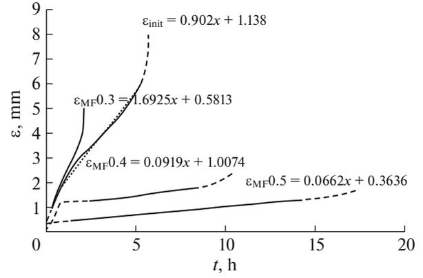
**Fig. 1.** Creep curves of polycrystalline lead in ( $\varepsilon_{\text{init}}$ ) initial state and ( $\varepsilon_{\text{MF}}$ ) under action of magnetic field with inductions  $B = 0.3, 0.4,$  and  $0.5$  T.
