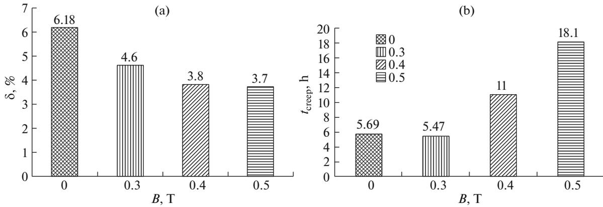
Fig. 2. Dependences of (a) the percentage of the relative residual elongation of the sample at fracture  $\delta$  and (b) the creep process time  $t_{creep}$  on  $B$ , T.
